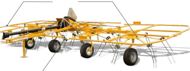
The transport lock on the TD190 can be released from the tractor seat, and the outside rotors can hydraulically fold to a 10.9-ft (3.3-m) transport width, making it convenient to quickly move from field to field.
