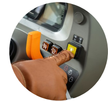
4. Independent rear PTO switch
