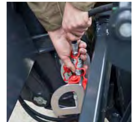
3 Plug in the hydraulic connection
