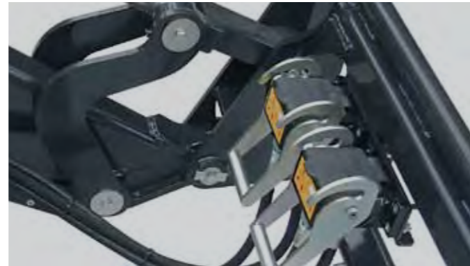
Tool Fix 2-way coupling for the 3rd and 4th control circuit.
