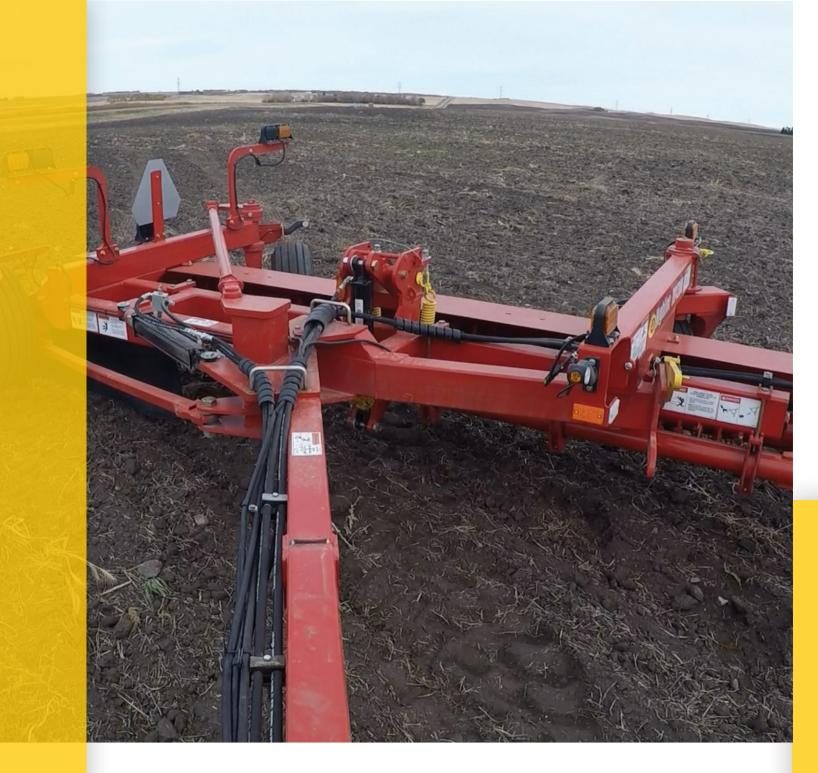
The RR 4300 rock rake is the perfect partner to the NT 60 and NT 78 rock picker! The RR 4300 rock rake makes fast work of moving rocks into a narrow row that can then be picked with the NT 60 or NT 78 rock picker. The stand-alone rock rake can keep moving while the rock picker is stopped to unload, resulting in more rock removed from a larger area in less time.
