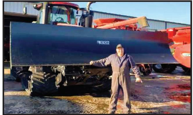
Keith showcases LEON high blade lift capabilities on this Case Model 375 Series Quadtrac. This feature is great for stacking and piling snow and silage.
