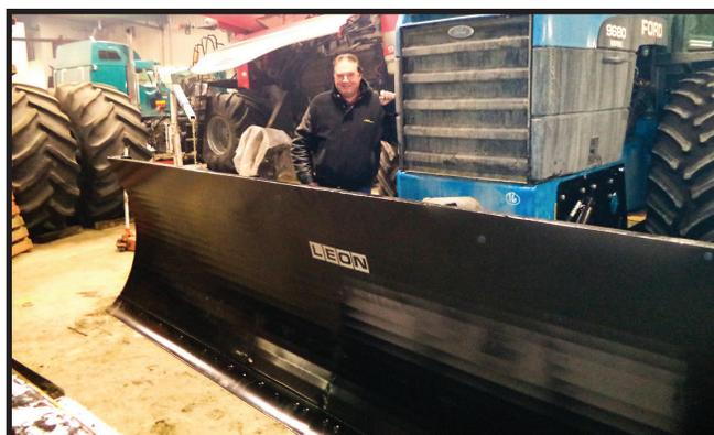
New Holland tractors from all eras continue to be a popular fit for LEON Dozer Blades. The LEON design was engineered to place minimum stress on tractor frames while providing a higher level of safety.
