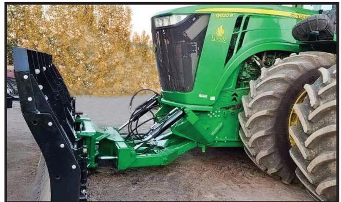
Powerful 'industrial strength' RAM Hydraulic Cylinders are strategically positioned on LEON Dozer systems to avoid exposure to debris when in operation.
