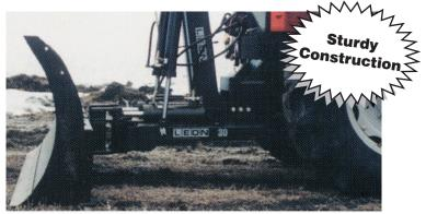
Sturdy Construction and Mounting is featured to insure these units stand up in the toughest of conditions. All push pressure is directed to the tractor drawbar area and is designed to place minimum stress on the tractor framework. All hydraulics included.
