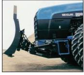
The tight fit frame construction and unique hidden hydraulic mounting allows the tractor to have a smaller turning radius. This is a must when you are working in tight spots.
