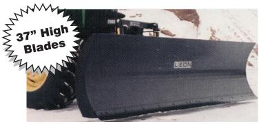
New High Definition Blades are 37" (94cm) high in 8 ft (2.44m) to 14 ft (4.27m) widths. The ripple formed blade insures clean roll off and roll break action to make pushing easier for the tractor.
