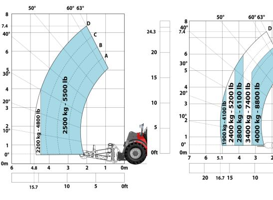
Machine on tyres with forks LC 600 mm Metric
