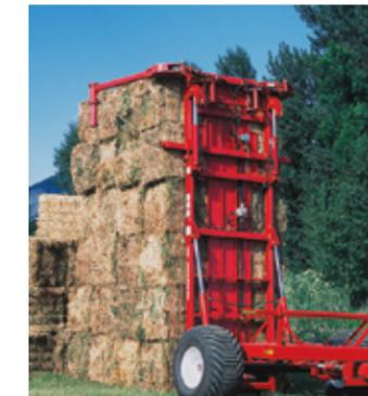
Once the bed is vertical, alignment arms are opened, and the 12SR is driven forward to remove the forks from under the stack.
