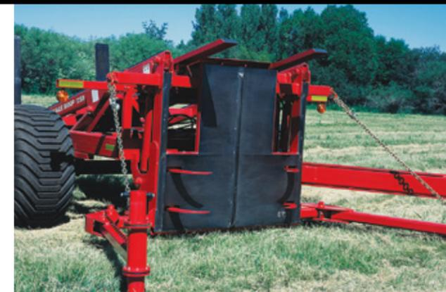
The Auto Align® system allows the operator to pick up bales in the same direction as the field was baled (12SR model shown).
