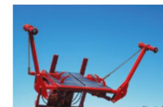
Grab hooks hold the first bale in place. Unique floating pipes on the alignment arms hold the second bale, to create the forward stair-step.
