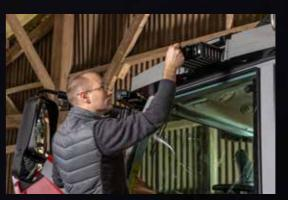
Easy access to remove the cab air filter for cleaning.
