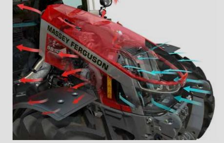
A new optimised airflow system improves engine cooling, which increases performance and boosts efficiency. Thanks to renewed wide grills, all radiators have full access to fresh air (thanks to the new design), providing maximum efficient cooling.
