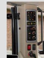
Accurate electronic control provides convenient and simple linkage operation. The ELC potentiometer is carefully positioned to the right of the operator for comfortable and easy use. providing precise control of implement depth as well as lifting and lowering the linkage.
