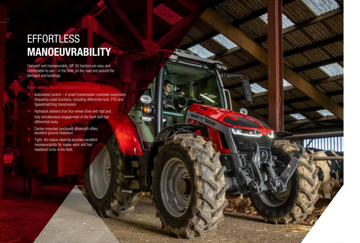
A new, stronger suspended front axle offers an industry-leading 4m turning radius. Working with the new 3t capacity front linkage, which can now lift an extra 500kg, it helps improve efficiency, enabling the tractors to use larger front-mounted equipment. Extra comfort is offered by the electronically-controlled hydraulic suspension, which uses two longer stroke cylinders and three accumulators to absorb shocks.
