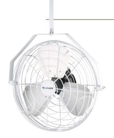
The HAF18 features a 1/15 HP totally enclosed, 115V, 0.9 amps motor. The variable speed motor can be adjusted accordingly to meet your requirements. It features open guard spacing for better air distribution and a hanging bracket. When suspended, fan can pivot up and down and swivel 360° for optimal control of air stream.
