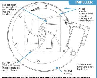
Voluted design of the housing and curved blades are continuously being loaded and unloaded, keeping a constant positive pressure at the discharge point. As the impeller turns, slurry is forced to the outer band area, which becomes larger as slurry approaches the discharge point. More slurry is being constantly added to the impeller blades as slurry moves away.
