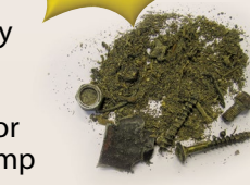
Actual tramp metal removed from magnet.
