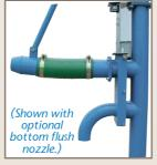
**Tapered-bore drive pulley** mounts to a 1% inch (44.5 mm) drive shaft with a greaseable flange bearing at the top of the drive tube.
