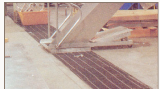
▲ Metal shavings drop into this grate-covered trough where a Patz Material Mover conveys them to a storage bin.
