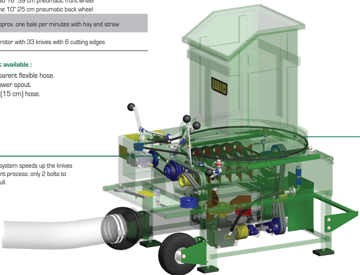
Revolutionary spacer system speeds up the knives rotation or replacement process: only 2 bolts to unscrew, no rods to pull.
