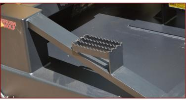
Step plate for easy entry into skid steer
