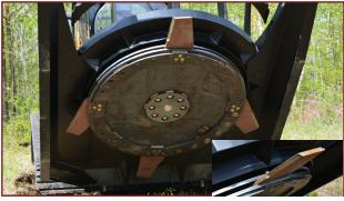
(2) Optional 4 Blade Assembly. Inset is close up of blade and dual carrier.
