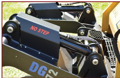
Two Independent Hydraulic Cylinders
