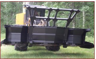
192 - Two hydraulic retractable wings adjust for transport and your environment\*
