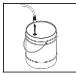
**STEP 1:** Remove detergent suction tube from soap container and insert into one gallon of fresh water. Use black soap nozzle with detergent injector. Pull trigger on spray gun and siphon water for one minute.
