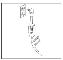
**STEP 3:** Connect to appropriate power supply. Push GFCI reset button.
