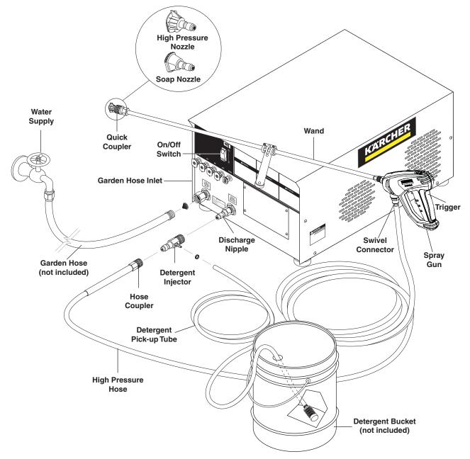
**Detergent Injector** - Allows you to siphon and mix detergents, when used with soap nozzle.
