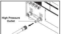
**STEP 6:** Disconnect the high pressure hose from high pressure outlet.
