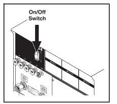
**STEP 4:** Turn machine on by pushing switch at front of machine.
