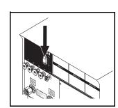
**STEP 2:** Turn off machine by pushing switch on front panel.
