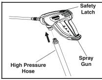
**STEP 1:** Attach the high pressure hose to the spray gun using teflon tape on hose threads. Use safety latch to prevent from opening.
