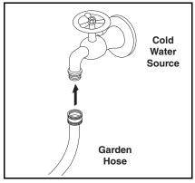
**STEP 1:** Connect garden hose to the cold water source and turn water on completely. Never use hot water.
