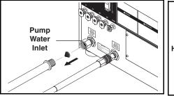
**STEP 5:** Disconnect the garden hose from the water inlet on the machine. Protect from freezing.
