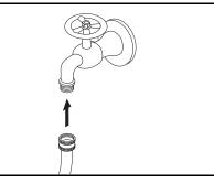
**STEP 2:** Connect garden hose to the cold water source. Before installing nozzle, turn on water supply and run machine, allowing water to flush through the system until clear.
