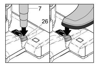
Brush height adjustment can be changed by foot or with the attachment tube.
