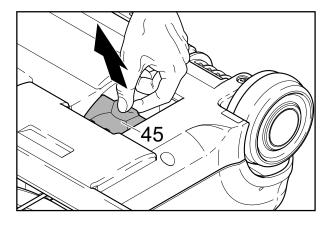
Check for a blockage in the swivel neck of the power head and under the yellow trap-door (45) on the bottom of the power head. Ensure that the passage between these two openings in the power head is clear.
