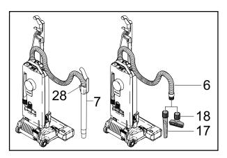
To use the attachment tube (7) or hose (6) put the machine in the upright position, then lift the tube from the machine and stretch out the hose until it locks. When the tube is returned to the machine, ensure it is pushed down over the projection (35) on the housing.
