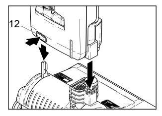
To dismantle, press the release button (12) and remove the dust bag housing (20) from the power head (9).
