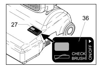
This vacuum cleaner has a brush jammed indicator (27). If the brush is jammed or overloaded the machine will automatically switch-off and the orange indicator shows in the display (36). If this occurs, unplug the machine and clear the obstruction.
