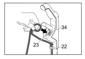
Finally insert the mains cable into the cable cleat (23). You can hear a "click" when the mains cable is fully inserted. To take off the mains cable push the button (34) next to the cable cleat (23) and remove the mains cable.
