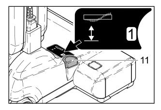
By pressing the button (11), the brush can be adjusted from position 1 (lowest setting) to 4 (highest setting) and back.
