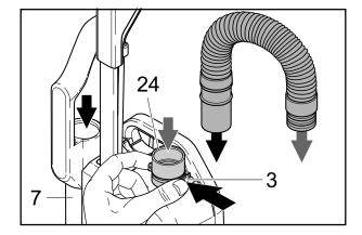
Fit the attachment tube (7) into the swivel neck (21) and then push the attachment tube handle (5) over the projection (35). Push the black end of the hose into the connecting tube (24) so that it clicks into place. The hose can be taken off by squeezing the retaining ring (3). The other end of the hose fits into the attachment tube (7) only one way.
