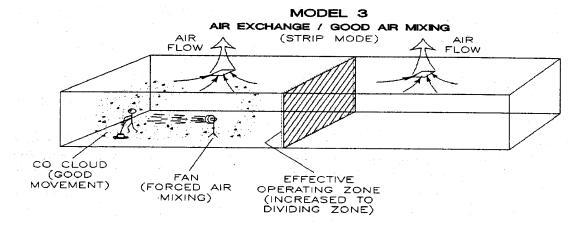
Notice the CO concentration and the Effective Operating Zone (Expanded to the Dividing zone) with air exchange and forced air mixing. The CO cloud is still concentrated on one side of the Dividing zone. Note the "Dividing Zone" shown above, this is the line where airflow changes direction. In Model 3, air changes are cut in 1/2 as little or no CO crosses the Dividing Zone to be exhausted.
