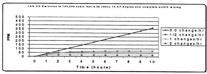
Based on the CO production rates shown above the TWA would be exceeded in a 100 x 500 x 10 foot (empty) space after 6 hours with 2 air changes per hour. (Assumes no additional CO exposure during 8 hour time period).
