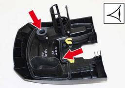
Check the condition of the seals between the appliance and the wastewater reservoir; replace if required.
