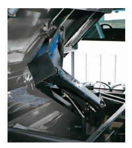
The power behind the Deuce is a double-acting Lo-Boy<sup>®</sup> hoist on a bayonet swivel. The additional double-acting power allows the Deuce to lift larger loads-up to 11 ton capacity!
