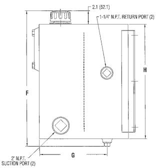
Note: Desired fill point determined by installer. Usable capacity limited by fill point and pump outlet port position.
