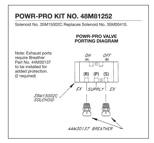
Note: This supplement to be used in conjunction with the original installation instructions. The new solenoid valve being used along with the addition of a breather in the exhaust port(s) is for added protection against contamination.
