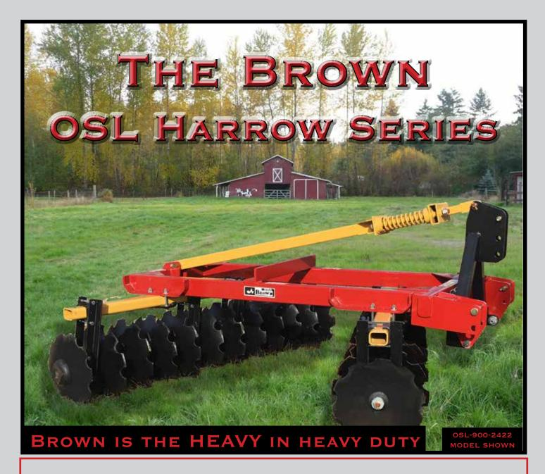
The Brown Offset Gang Disc Harrow is a heavy duty all purpose harrow. All units standard with heavy duty welded tube frame, trunnion mounted triple-lipped sealed steel ball bearings and high strength forged 1-1/8" gang axles, mid-mount weight rack for suitcase weights. Seven Gauge (0.177", 4.5MM) notched disc blades.
