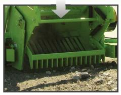
Grate & reel with 3/8" thick square batts and 11/2" spacing
