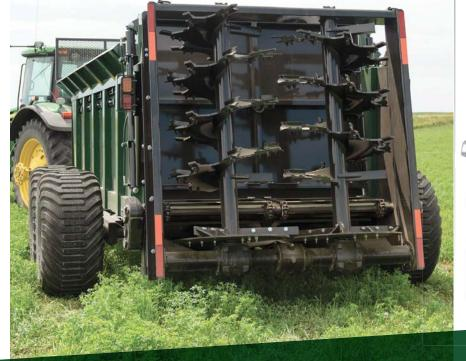
Creates less field compaction and utilize a lower loading height when you choose the flotation tires instead of our standard used military tires.
