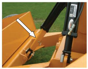
Figure 10. Lift cylinder mechanical safety stop.
