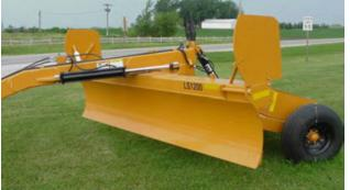
Figure 6. Box ends locked in up position.
