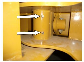
Figure 13. Steering pivot zerks (2).
