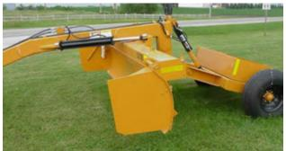
Figure 7. Box ends locked in down position.
