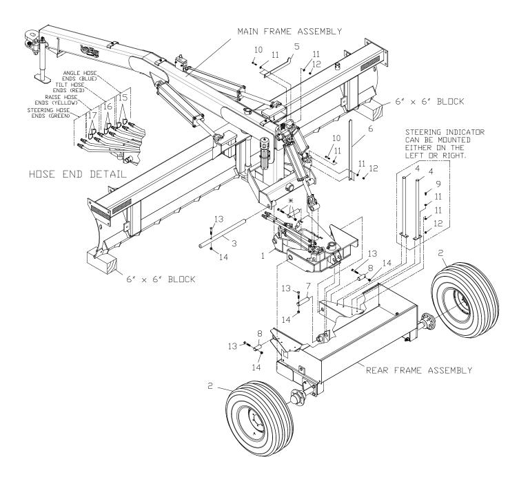
Figure 4. Rear Steer Grader Kit Assembly
