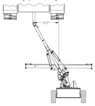
Figure 8. Steering Offset Operation.
