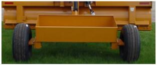
Figure 9. Sandbox on rear frame assembly.
