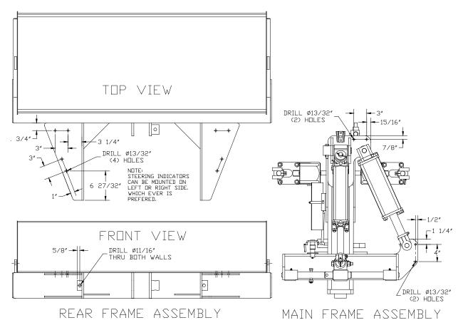
Figure 3. Rear Steer Grader Kit New Hole Locations for Indicators.
