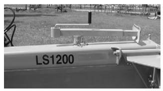
Figure 11. Jack storage on moldboard.
