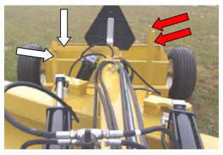
Figure 5. Level and Steering Indicators
