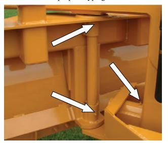
Figure 11. Moldboard pivot (2) and tilt (1) zerks.
