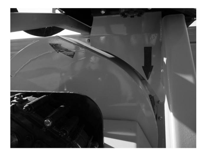
Rotate fan housing either left or right completely until it hits the stops to use the side discharge.
