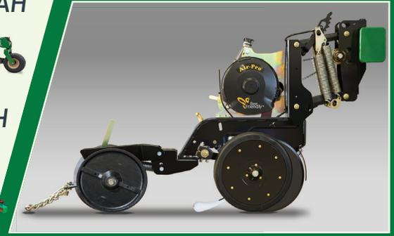
The 25 Series row unit utilizes ductile cast parallel arms for long-term row unit stability. 15", 4mm blades turning on 205 triple-lip sealed bearings ensure long life and accurate seed depth. Blades are offset 1/2" to slice residue and form a perfect seed trench.
