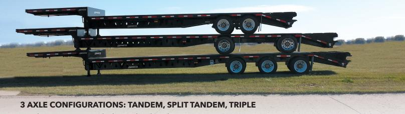
Air ride suspension is standard on triple axle trailers
