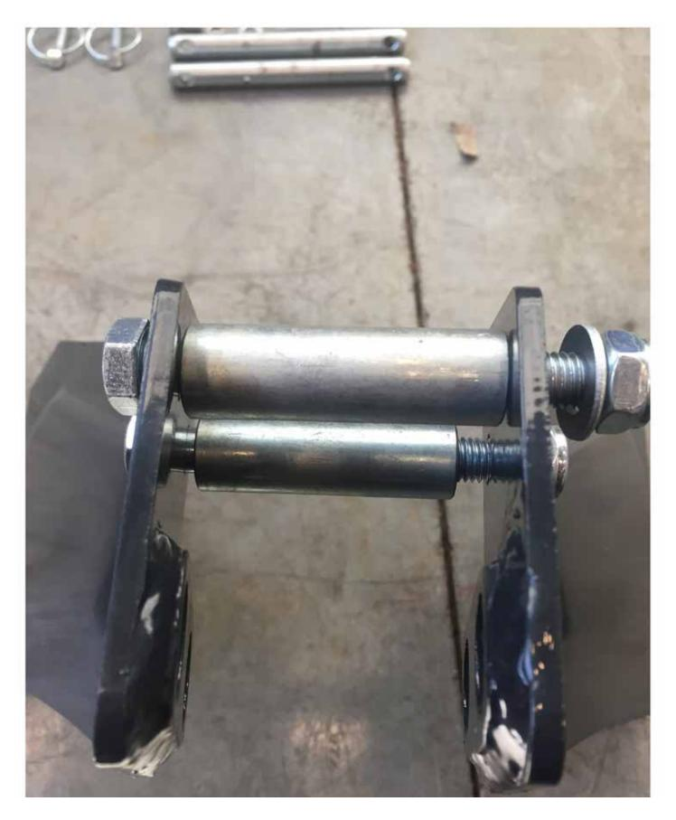
•When assembling the top of the 3 point hitch, keep all of the hardware loose until it's mounted. Tighten the bottom 8 12 mm bolts first, then the top 2 12mm bolts, and the 2 8mm bolts that hold the cover plate last.
