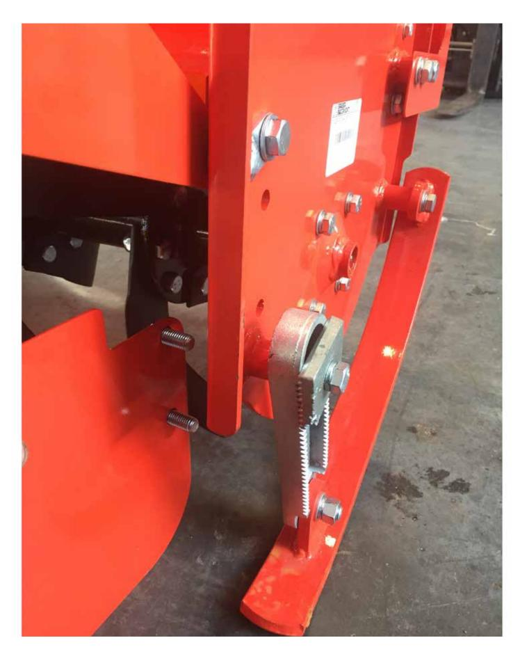
•When installing the side guards beside the tailgate, the bolt head must be inside the tiller case and nuts must be on the outside or the blades will hit the bolt.
