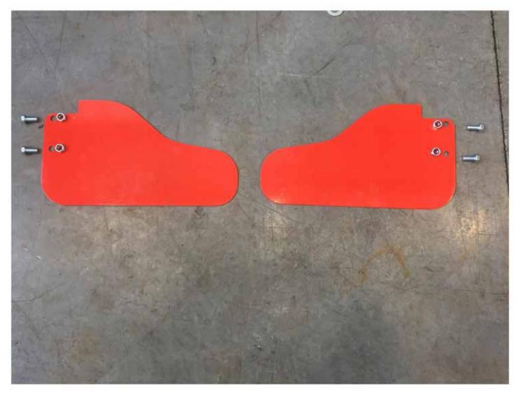
•When installing the side guards beside the tailgate, the bolt head must be inside the tiller case and nuts must be on the outside or the blades will hit the bolt.
