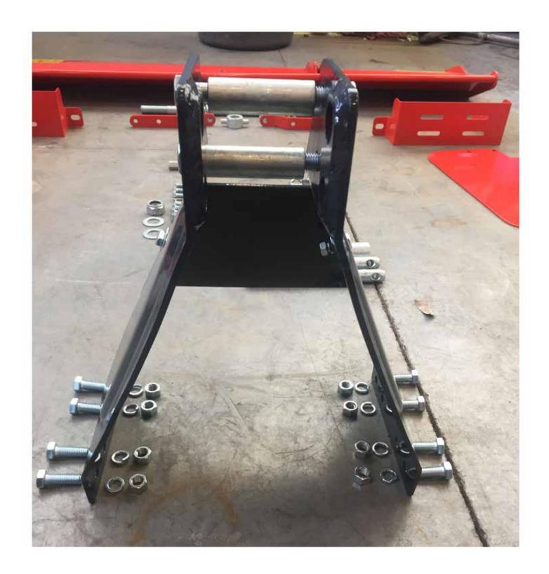
•When assembling the top of the 3 point hitch, keep all of the hardware loose until it's mounted. Tighten the bottom 8 12 mm bolts first, then the top 2 12mm bolts, and the 2 8mm bolts that hold the cover plate last.
