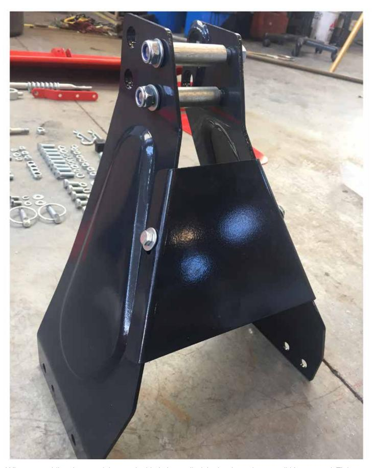
•When assembling the top of the 3 point hitch, keep all of the hardware loose until it's mounted. Tighten the bottom 8 12 mm bolts first, then the top 2 12mm bolts, and the 2 8mm bolts that hold the cover plate last.
