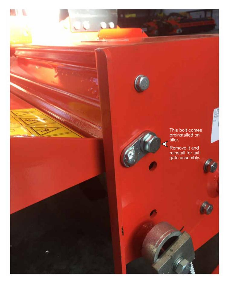
•When installing the tailgate, the bolts for the pins are already on the machine. They simply need to be loosened and pulled out.
