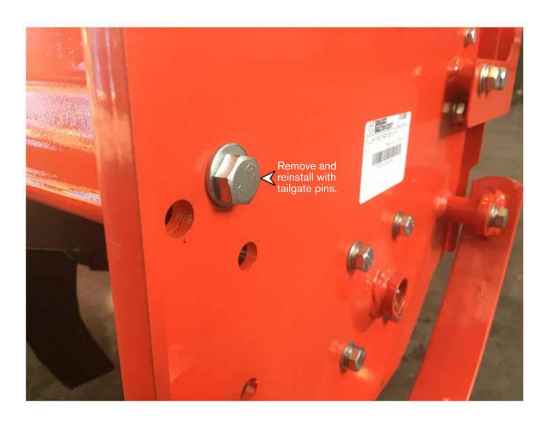
•When installing the tailgate, the bolts for the pins are already on the machine. They simply need to be loosened and pulled out.
