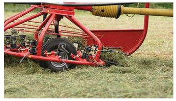
The centrifugal force-controlled, horizontal tines self adjust to field contours as they float through stubble to cleanly pick up crop, providing faster working speeds with little risk of contamination when tedding and raking.
