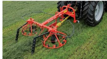
The HayBob 300 provides efficient tedding and quality centerdelivery raking. Adjustable swath boards produce neatly formed windrows and may be offset to form a double row in three passes.
