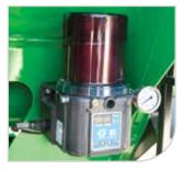
Auto-greaser system for automatic application at more frequent intervals for consistent lubrication of track undercarriage
