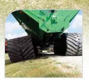
Tracks equalize to follow altering terrain – each track independently cambers to follow ground contours for optimum flotation and minimum compaction
