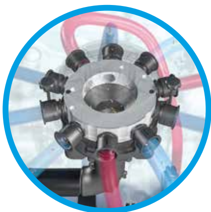
Distributor with switched tramlines
