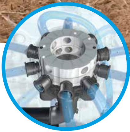
Distributor in sowing mode
