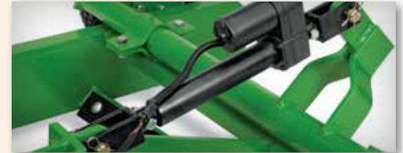
Optional electronic actuator on the LP10 Series connects to a 12-volt power supply, allowing you to raise the implement quickly and easily from the comfort of your seat.
