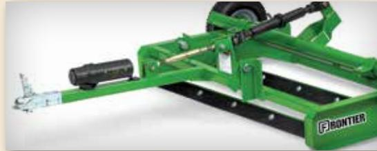
Pull-type LP10 Series Land Planes are a perfect fit for utility vehicles equipped with a 1-7/8-in.-diameter (4.76 cm) ball hitch.
