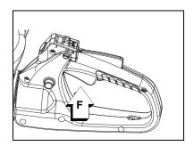
2. Stop Switch Move stop switch (A) to STOP position.
