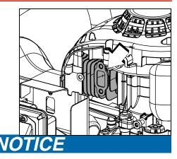
Never use a metal tool to scrape carbon from the exhaust port. Do not scratch the cylinder or piston when cleaning the exhaust port. Do not allow carbon particles to enter the cylinder.
