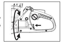
Note: The throttle trigger will not operate when the throttle handle is not fully locked into position.
