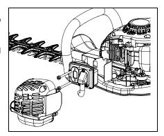
3. Use a wood or plastic scraping tool to clean deposits from cylinder exhaust port.
