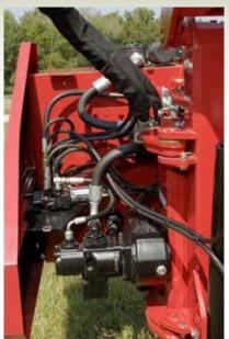
All RMB models offer self-contained, fully independent hydraulic systems with twin pumps for optimum cutting performance.
