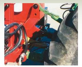
Fast attachment to your tractor is acheived with the Cat. Il Standard and Cat. Il & Ill Quick Hitch.
