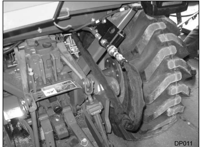
Figure 17. Tractor Hose Connection - Backhoe Removed (Typical)
