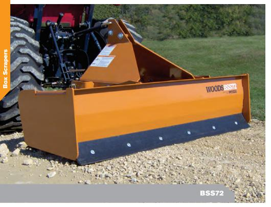
Tackle the toughest spreading and grading jobs with Woods and Gannon brand box scrapers. From the reinforced steel A-frame to the tough, reversible cutting edge and replaceable scarifiers, our box scrapers deliver exceptional durability and versatility.
