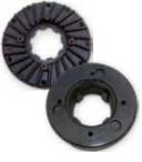
The shredder drive is protected with either a 24,000 lbs inch overrunning disc clutch (not available on S30CD) or a 30.000 lbs inch overrunning automatic clutch, which is made completely of metal and disengages when torque limit is reached. To reengage, tractor PTO speed is reduced to match that of the gearbox input shaft.
