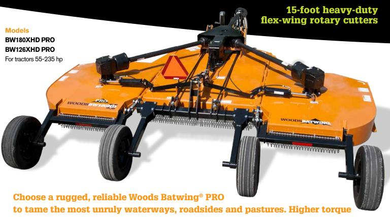
capacity, a deep 7-gauge deck, and innovative wing design ensure you'll mow more material in less time.
