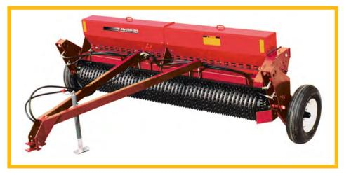
hydraulic transport with (2)  $7.60 \times 15$ " tires. All models include warning light kits. Use the one seeding method that you can depend on to produce a top stand time after time...a Brillion Sure Stand Alfalfa Seeder.
