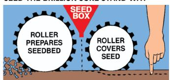
Front rollers crush lumps, press down small stones, and form a firm seedbed. Precision seeding devices meter out the seed onto the well prepared seedbed. The rear rollers split the shallow ridges formed by the front rollers and gently firm the soil around the tiny seeds. All seeds are planted at fingernail depth for top germination and fast emergence.
