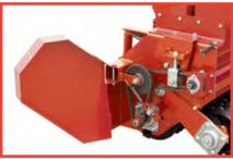
The seeder drive mechanism has been updated to utilize an all roller chain drive train with ball bearing idlers that ensure proper chain tensioning. Number 40 roller chain is used throughout to maintain
