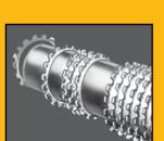
High Strength Rollers. Roller wheels are made of 34,000 lb. tensile strength gray iron, cast in Brillion's modern electric foundry under strict quality control. These wheels (2" wide) prepare a perfect seedbed and control seeding depth. Wheel notches
