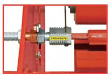
The adjustment of the Micro-Meter has been made user friendly by implementing a new calibration collar and pointer system that requires the use of two wrenches that are provided with the seeder. Seed rates charts are provided to give starting rates for a variety of seeds.
