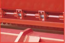
The front Micro-Meter box is designed for the precision metering of legume style seeds such as Alfalfas and Clovers. The exact spacing of the Micro-Meters provides uniform seed distribution for optimum aermination.
