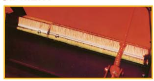
**Brush Agitators -** keep the seed flowing at a positive, accurate rate and provide instant shut-off the moment the seeder is stopped; prevents seeding "skips" and bunching of seeds.
