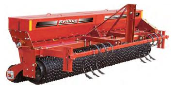
SSBP12 equipped with optional wheel track removers.
