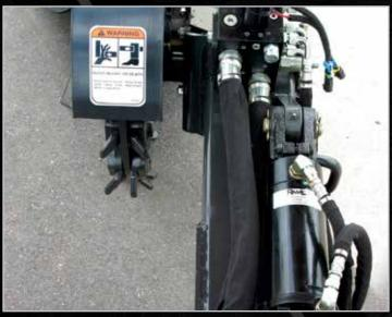
Offset wheel allows operator better visibility. Quick Stump-Away's hydraulic motor powers the 1/2" steel cutting wheel to an impressive 1100 rpm.
