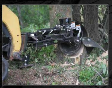
Up to 1,100 RPM cutting wheel speed to grind stumps in no time!
