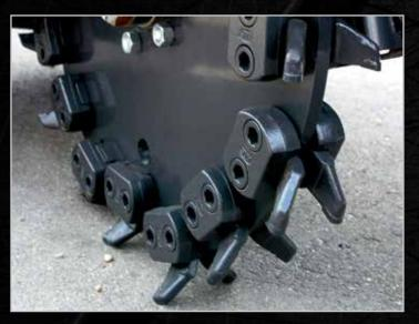
Carbide teeth aggressively chew through any size stump with little wear.
