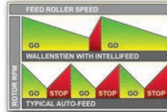
The optional fully programmable, IntelliFeed monitors the rotor's rpm, slowing the rollers' speed as needed. IntelliFeed continues the chipping at a volume that best matches its rpm.
