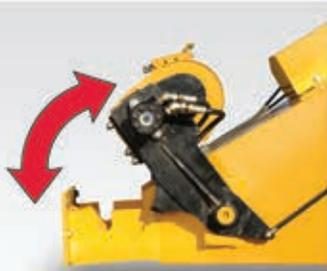
Lift assist for servicing using gas shocks.
