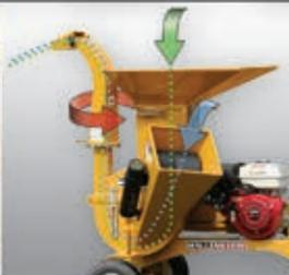
Chipper & Shredder use the same 360° exit chute
