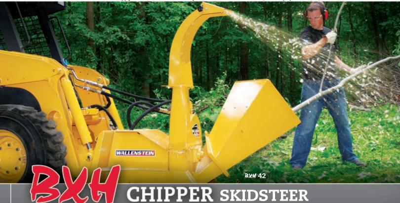
Get the most out of your equipment with the practical BXH 42 **Skidsteer Mounted** Wood Chipper. The hydraulically driven BXH 42 is powered directly from the skidsteer's external ports, providing plenty of chipping action.
