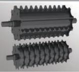
Hydraulically driven dual active rollers
