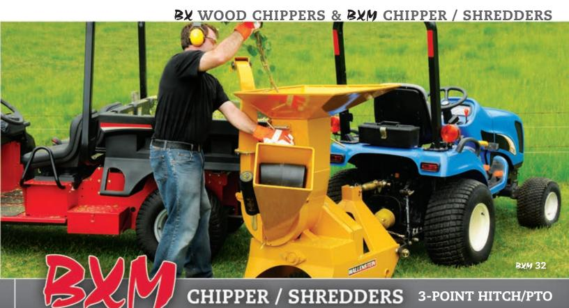
Directly connected to your tractor's PTO, power is transferred straight into chipping / shredding action - quickly turning limbs, branches or debris up to 4" in diameter into valuable chips or mulch.
