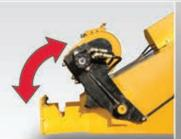
Lift assist for servicing using gas shocks.
