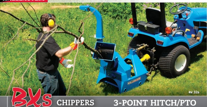
Directly connected to your tractor's PTO, power is transferred straight into chipping / shredding. The self-feed hopper automatically pulls the branches in as it chips.
