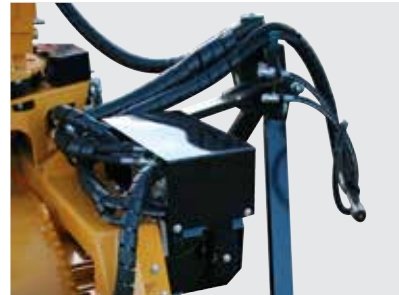
Kit of electric directional control valves to control hydraulic functions.
