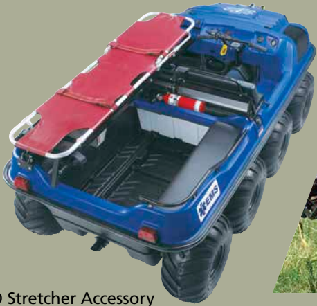
ARGO Stretcher Accessory fits ARGO 8x8 700 HD and 750 HDi models and is designed for Ferno Stretcher #9.
